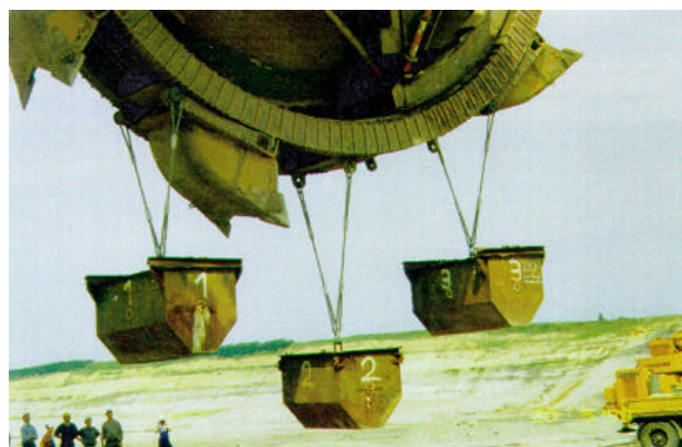
Picture 1: Records of load and stress data at a lignite excavator, calibration
