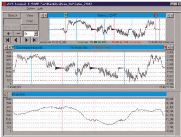
Picture 9: Sequential Extremes with Time and Master/Slave Function. Presented as amplitude progression with master and slave channel.
